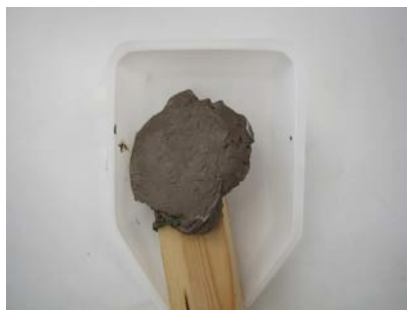
Figure 20. Thickened formula B 1 stuck to the piece of wood used for mulling.
