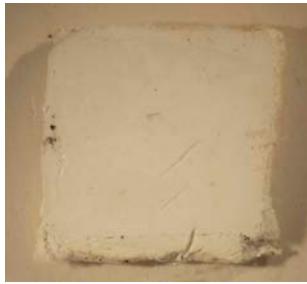
Figure 13. Multiwax® W-445 with titanium white; 41% pigment by weight
