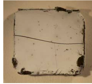
Figure 11. Unbleached beeswax and Elvax 150 (5:1) with raw umber; 32% pigment by weight
