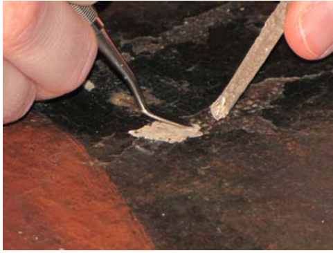
Figure 2. Compressing wax into loss with heated dental tool.
