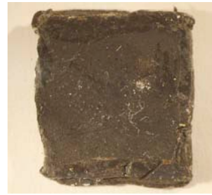
Figure 14. Multiwax® W-445 with raw umber; 21% pigment by weight
