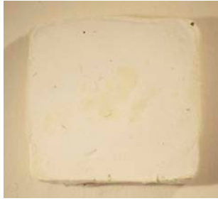
Figure 10. Unbleached beeswax and Elvax 150 (5:1) with titanium white; 46% pigment by weight
