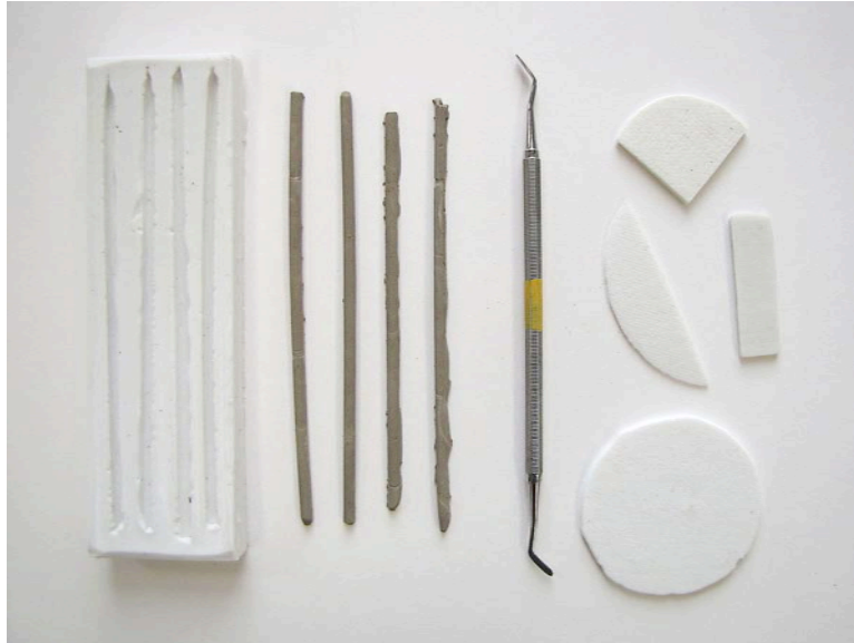
Figure 1. From left to right: silicone mold, four pigmented wax/resin sticks, dental tool, and pre-made Dow RTV 3110 silicone rubber molds with canvas texture impressions (cut to various sizes).
