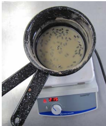
Figure 19. Insoluble resin floating in waxes of formula B
