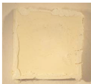
Figure 7. Unbleached beeswax with titanium white; 38% pigment by weight
